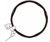
Press the remaining sections of the seal.
